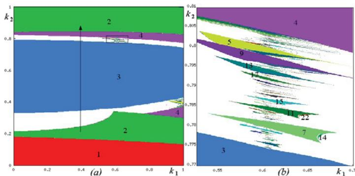
Figure 3: Two-dimensional bifurcation diagram in the  $(k_1, k_2)$ -parameter plane for  $n = 23$  (a), and its enlarged part (b).
